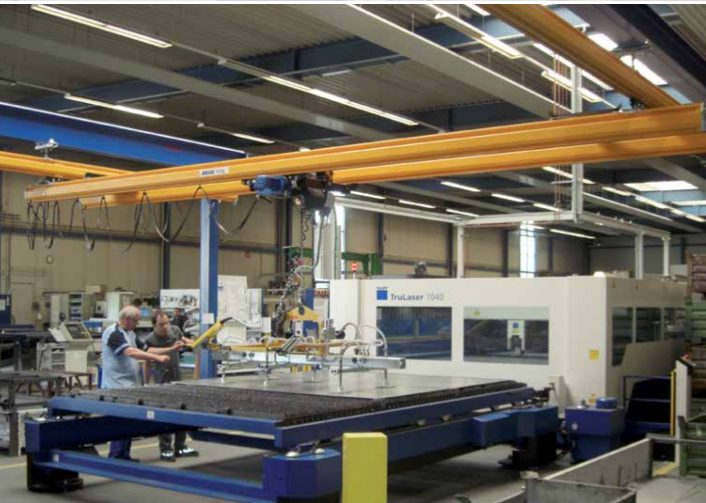
Two-bridge suspension crane system with electrical friction drive and a vacuum lifter VacuBoy
