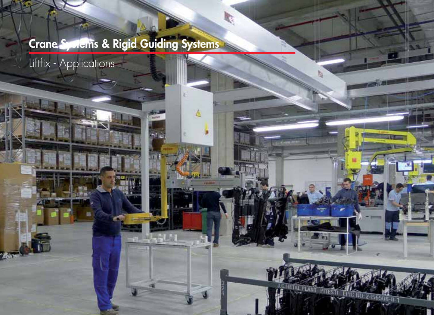
Liffix with mechanical gripper for handling seat frames for automobile industry
